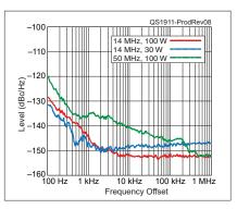
Figure 8 — Spectral display of the Yaesu FTDX101D transmitter output during phase-noise testing. Power output is 100 W on the 14 MHz band (red trace), 30 W on the 14 MHz band (blue trace), and 100 W on the 50 MHz band (green trace). The carrier, off the left edge of the plot, is not shown. This plot shows phase noise 100 Hz to 1 MHz from the carrier. The reference level is –100 dBc/Hz, and the vertical scale is 10 dB per division.
