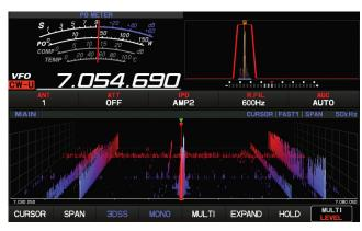
**Figure 2** — Same as Figure 1, except we have tapped the **3DSS** on-screen button and now have a three-dimensional view with time marching out the back of the screen, instead of the waterfall. This way, you can see what happened before, as well as what's happening now.
