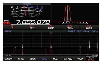
**Figure 1** — The Yaesu FTDx101D display showing a single panadapter, with waterfall below, for 50 kHz of the 40-meter band centered on the frequency tuned by VFO A. The "filter function display" at the upper right shows the received passband with the received signal within. The spectrum span can be adjusted from a width of 1 kHz to 1 MHz in 10 steps.
