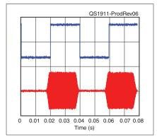
Figure 6 — CW keying waveform for the Yaesu FTDX101D showing the first two dits in full-break-in (QSK) mode using external keying and the default rise time setting. Equivalent keying speed is 60 WPM. The upper trace is the actual key closure; the lower trace is the RF envelope. (Note that the first key closure starts at the left edge of the figure.) Horizontal divisions are 10 ms. The transceiver was being operated at 100 W output on the 14 MHz band.
