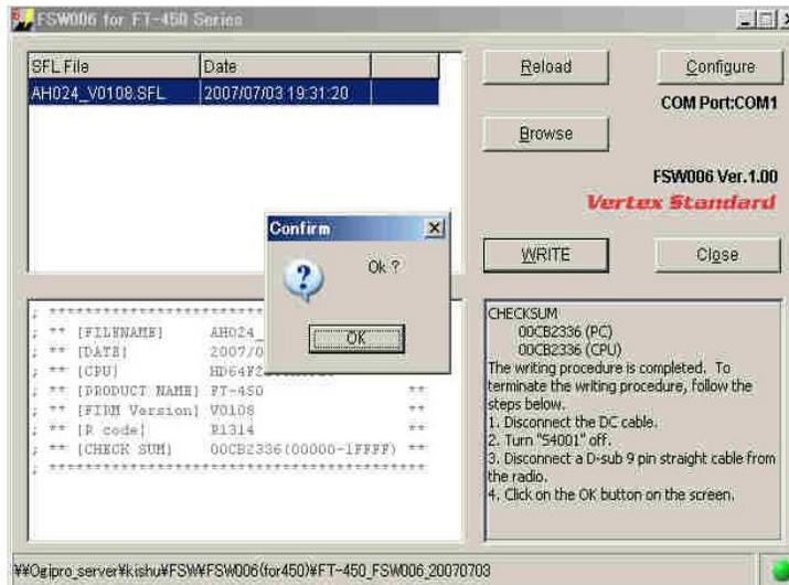
9. Disconnect the DC power cable and then remove the DB9 serial programming cable.
