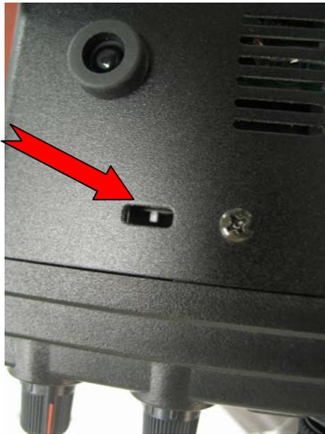
3. Connect the serial straight through programming cable, DB9F to DB9F, connector to the serial port COM1 in the back of your computer. Plug the DB9F connector to the CAT connector on the FT-450. You may also use a USB to serial adaptor if the DB-9 (RS-232C) serial port is not available on your computer.
