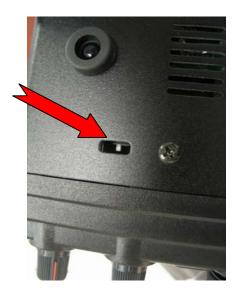
3. Connect the serial straight through programming cable, DB9F to DB9F, connector to the serial port COM1 in the back of your computer. Plug the DB9F connector to the CAT connector on the FT-450.
