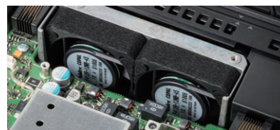
Thermostatically-controlled Dual Internal fans
