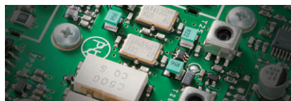
■ 3 kHz and 15 kHz Roofing Filters
