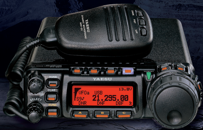
Ricetrasmittitore All Mode HF/50/144/430 MHz 100 W
