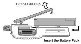
☐ To remove the battery, turn the radio off and remove any protective case. Slide the **Battery Pack Latch** on the bottom of the radio toward the front panel while sliding the battery down about 1/2 inch. Then lift the battery out from the radio while unfolding the Belt Clip.
