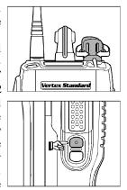
**MONITOR** button more than 2 seconds (or press the **MONITOR** button twice) to quiet the noise and resume normal (quiet) monitoring.
