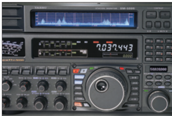
Figure 4 — Close-up of the main display and SM-5000 station monitor screen. To the left of the frequency display is information about the status of antenna, attenuator, filter, preamp, roofing filter and AGC settings for each receiver.
